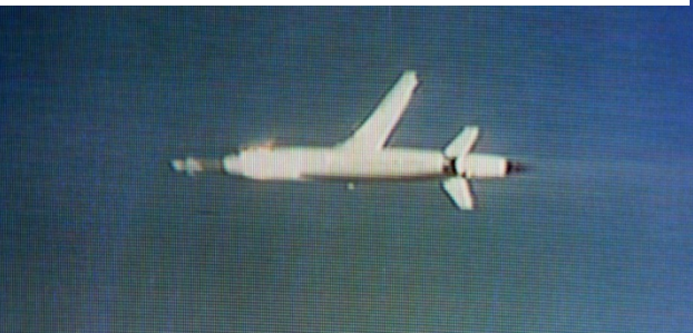
12 June 1980, shows the DAST-1 (Serial #72-1557) immediately after it lost its right wing after suffering severe wing flutter.
