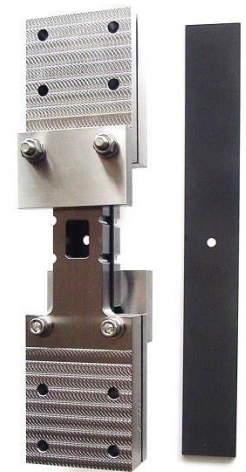
Open-hole compression fixture for monolithic composites
