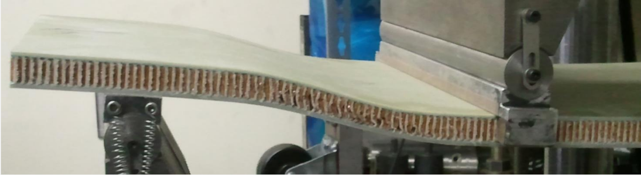
Core failure in outer region
