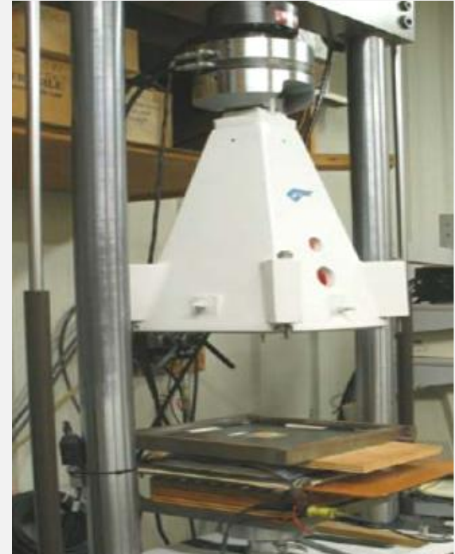
12 in. x 12 in. test panel 22-kip test machine (Gougeon Brothers, Inc.)
