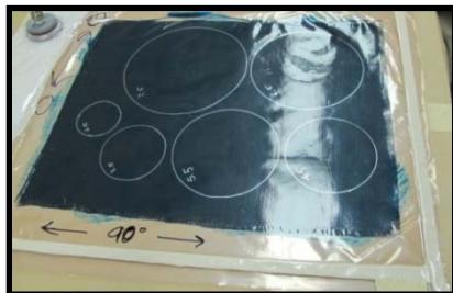
Wet lay-up resin impregnation
