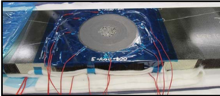
Scarfed panel ready for repair
