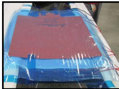
Heat Blanket Application
