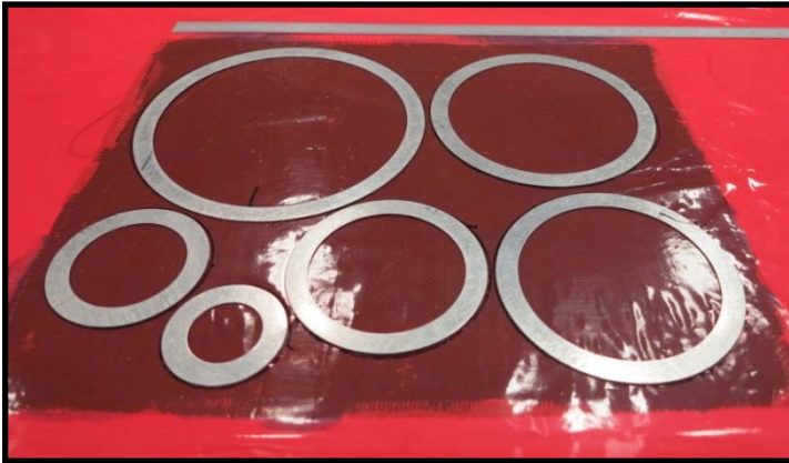
Wet lay-up ply impregnation
