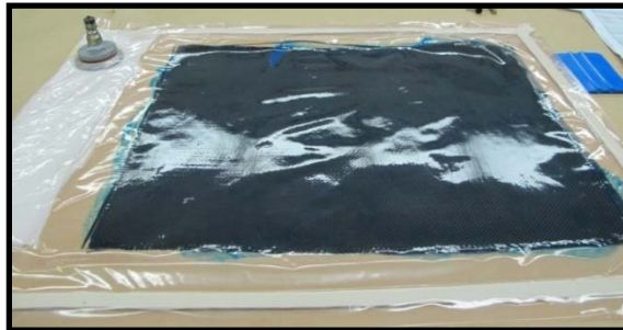
CACRC Repair Element Masking in Preparation for Scarf Sanding
