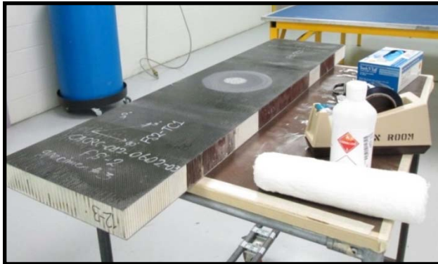
Element scarf sanded in preparation for repair
