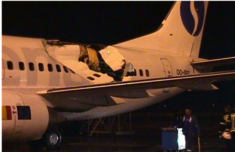
In-Service Damage, Courtesy Eric Chesmar, UAL [1]
