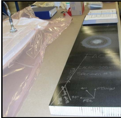
Repair Element Scarf Sanded in Preparation for Repair
