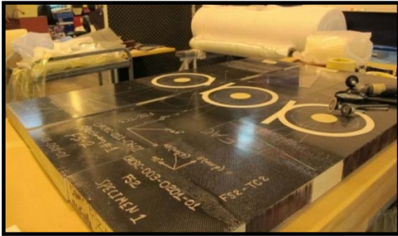
CACRC Repair Element Masking in Preparation for Scarf Sanding
