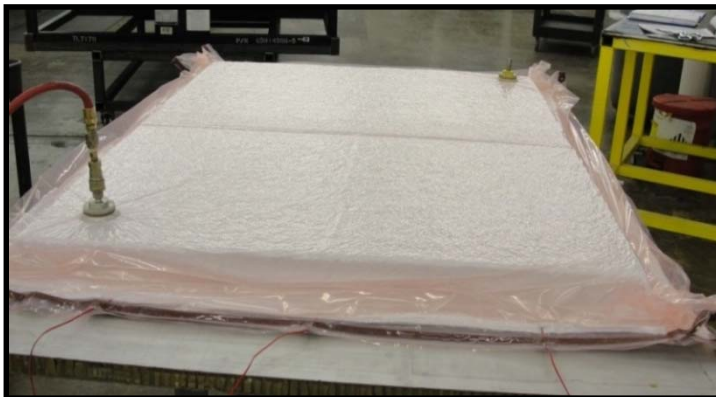
Repair Element Drying
