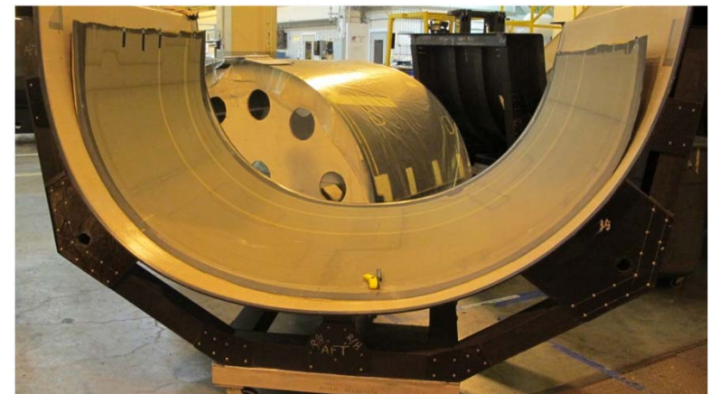
Complete Overhaul of a Composite Fan Cowl
