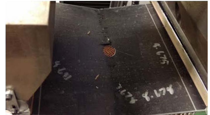
Failure of specimen with 1 in. hole
