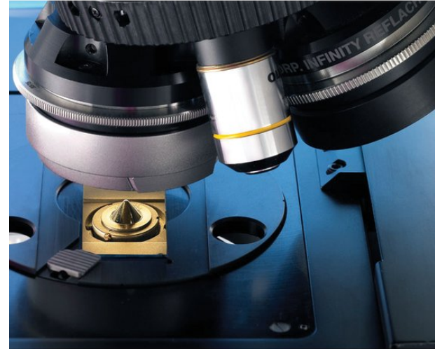
Spatial resolution achievable with the Slide-On TipATR Objective (Photosist target. Latter profile <5 \mu\text{m} wide)
