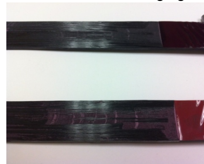
60001 polyester peel ply, sanded with environmental aging
