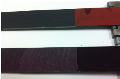
Nylon peel ply, as tooled no environmental aging
