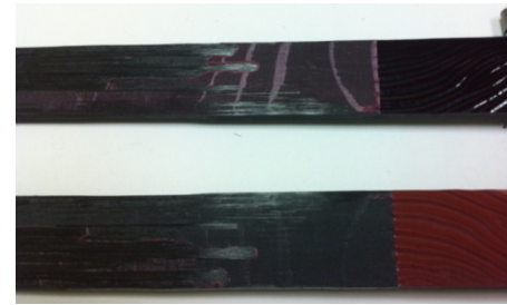
Nylon peel ply, sanded no environmental aging
