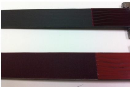
60001 polyester peel ply, as tooled with environmental aging
