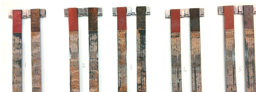
Freekote_single side contamination
