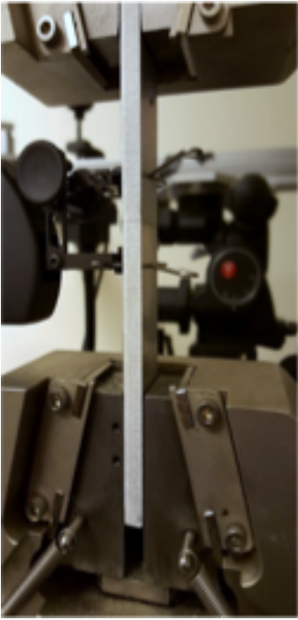
Butt joint being tested on an Instron load frame
