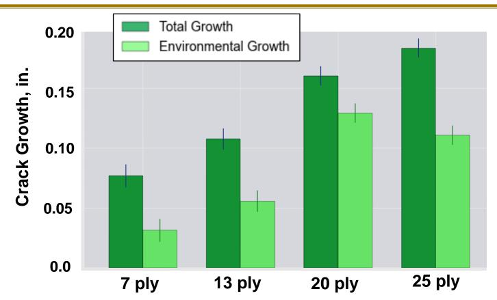
Increasing adherend thickness (and flexural modulus)...
