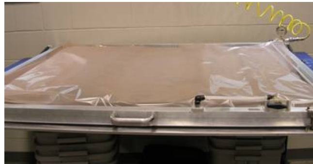
Core Potting, vacuum application
