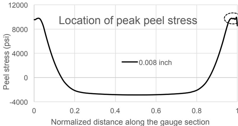
Peak peel stress vs. bondline thickness
