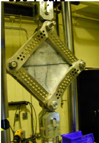
Picture Frame Shear Test Set-Up
