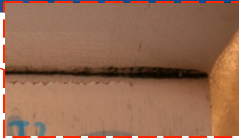
Load 2: Broken Shear Ties at 9 Locations (3 x 3 Frames)
