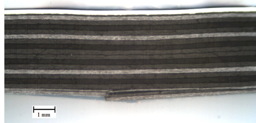
Damage to 16-ply panel by 12.7 mm radius tip.
