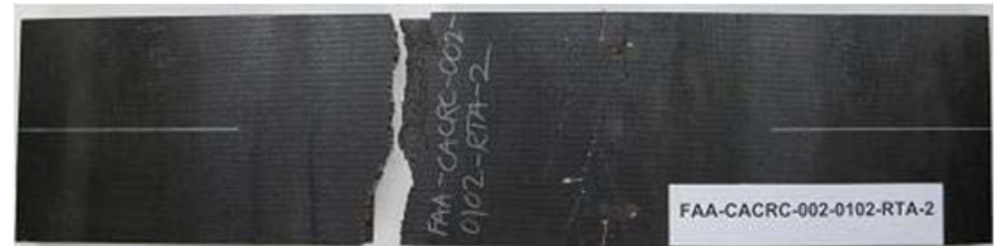
Typical Failure Mode – Undamaged beams
