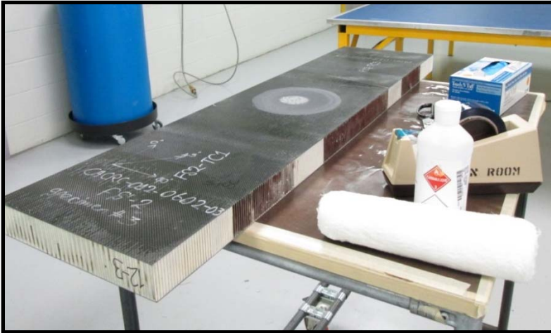
Element scarf sanded in preparation for repair
