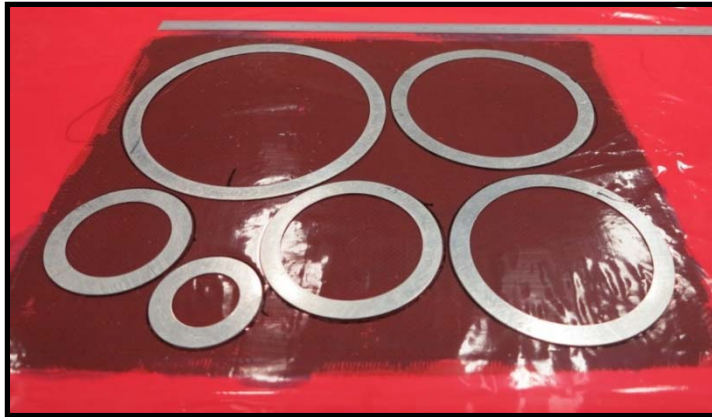
Wet lay-up ply impregnation
