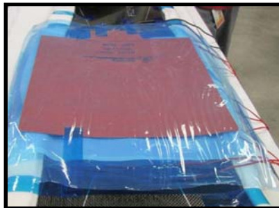
Heat Blanket Application
