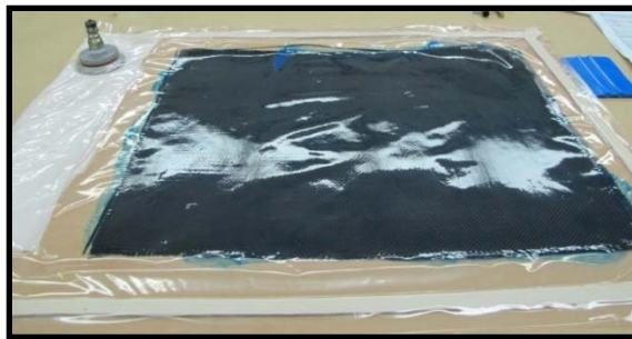
CACRC Repair Element Masking in Preparation for Scarf Sanding
