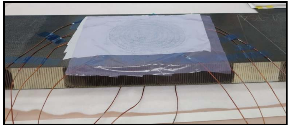
Wet lay-up repair bagging in preparation for cure
