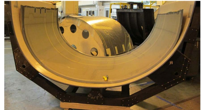
Complete Overhaul of a Composite Fan Cowl
