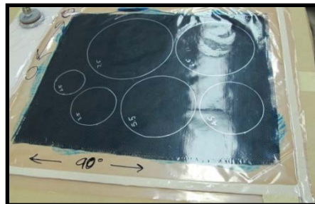
Wet lay-up resin impregnation
