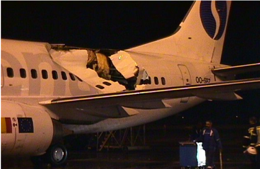
In-Service Damage, Courtesy Eric Chesmar, UAL [1]
