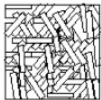
Quasi-isotropic discontinuous plate
