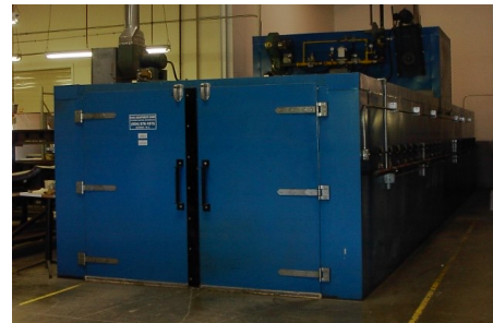
Three Curing Ovens 8'x 16' & 5'x 8' - 500°F; 9'x 40' - 375°F
