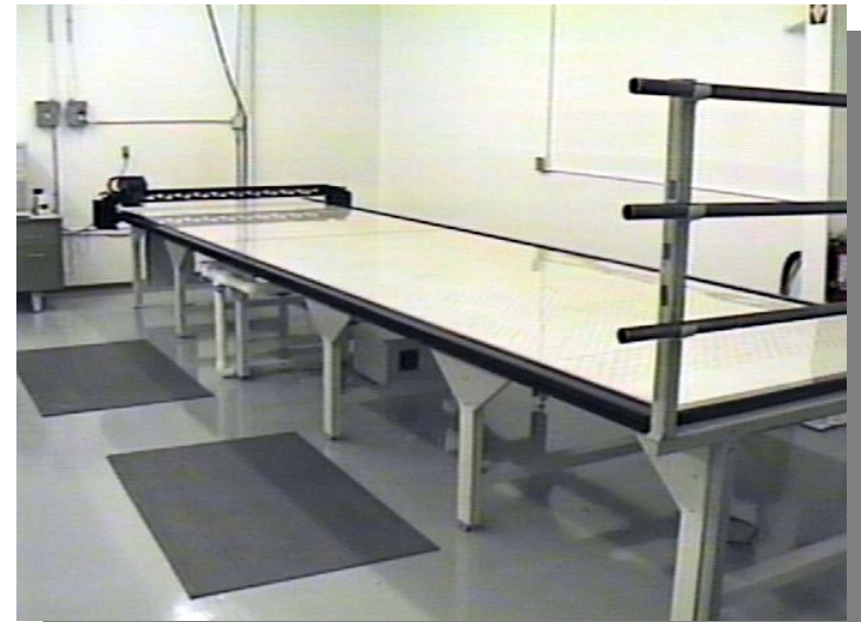
Autometrix - Automated Kit Cut Machine Automated Material Shape and Orientation Nesting Interfaces with CATIA and IGES Data
