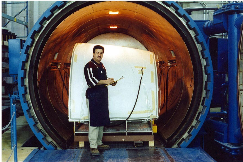
Two Full Temperature Range Autoclaves Baron 9'D x20' - 450°F, 150 psi Baron 4'D x7' - 450°F, 90 psi Automated Cure Cycle & Recording
