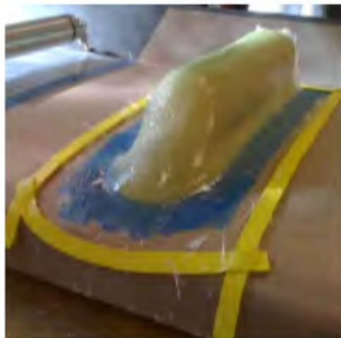
Figure 104 Lay-up of Fiber Glass Plies
