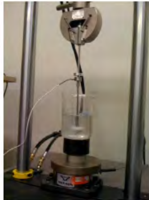
Testing for viscous force effects
