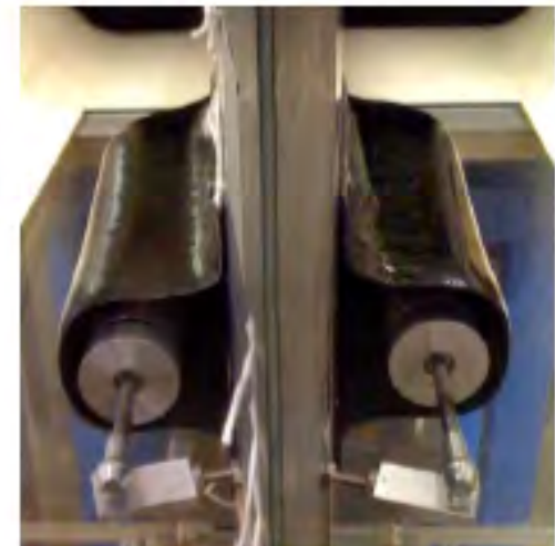
Figure 109 Both Dampers Mounted on the Structure
