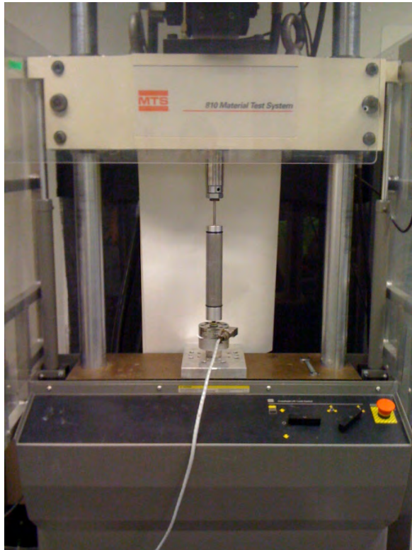
Damper in the Instron Machine
