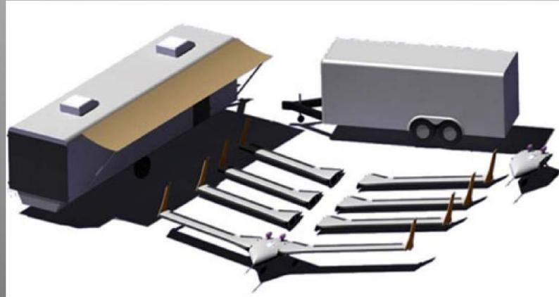
The X-56 aircraft system consists of two center-bodies, four wing sets, a ground control station, and a storage trailer.
