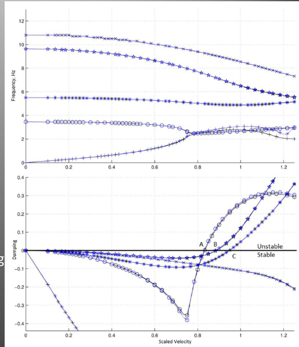
Natural frequencies and damping values as a function of scaled velocity.
