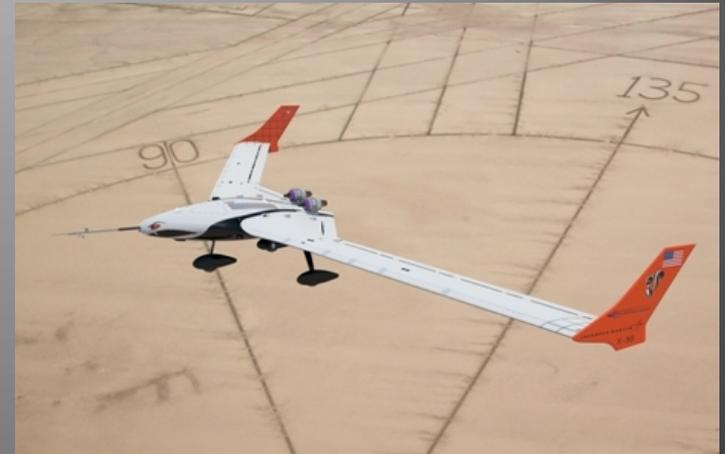
The X-56A Multi-utility Aeroelastic Demonstration (MAD) is an innovative modular unmanned air vehicle designed to test active flutter suppression and gust load alleviation.
