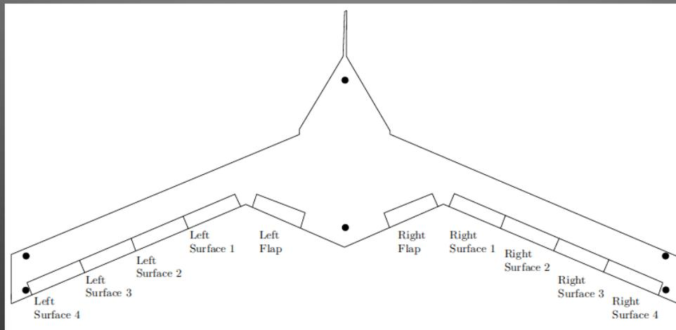
Control surfaces and accelerometers of the X-56 aircraft. Accelerometer locations are indicated with large dots. Control surfaces are labeled.
