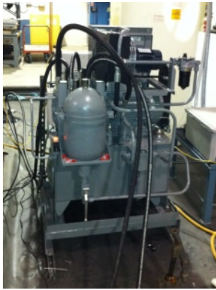
Hydraulic Power unit
