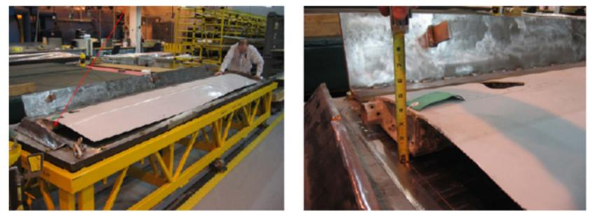
Utilizing tooling with incorrect contours, during the repair, caused a warp condition on the spar
