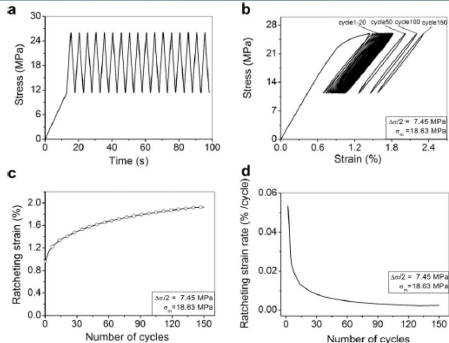
Fig. 3. Uniaxial ratchetting test of ACF: (a) stress control diagram; (b) stress-strain relationship; (c) ratchetting strain evolution; (d) ratchetting strain rate evolution.
