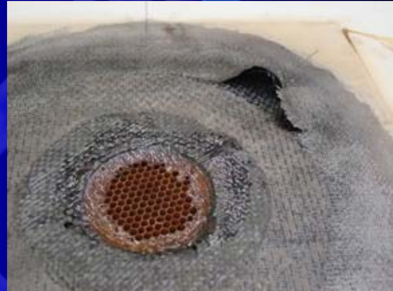
Laminate failure at high temperatures
