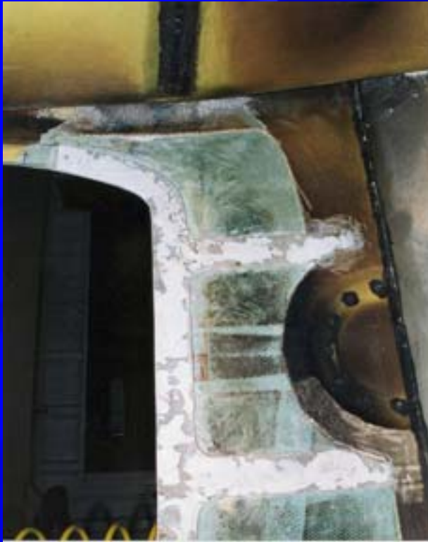
Laminate failure at high temperatures
