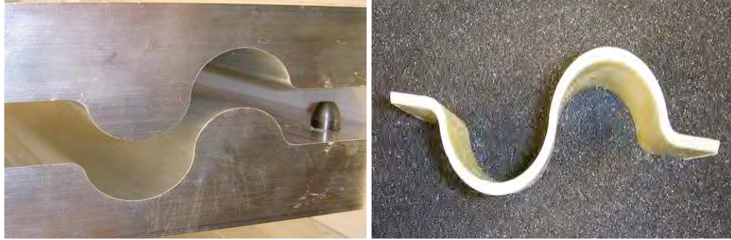
Figure 3. Matching molds and cured corrugated specimen 10 .
