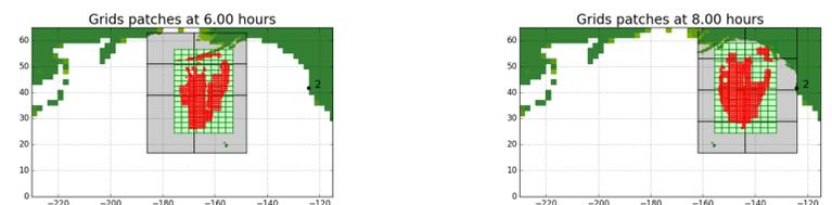
Grid patches when focusing on waves arriving between 11.75 and 12.5 hours after tsunami:
