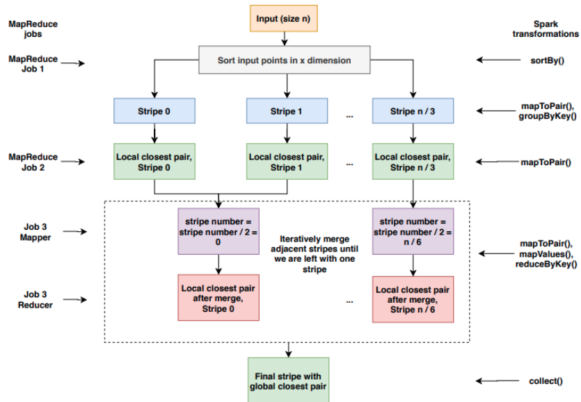
Figure 3.3: MapReduce and Spark closest pair of points algorithm
