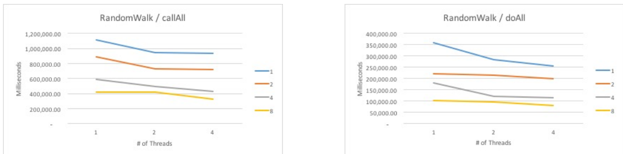
Figure 4.16: The effect of number of threads on callAll and doAll executions in large scale RandomWalk application.
