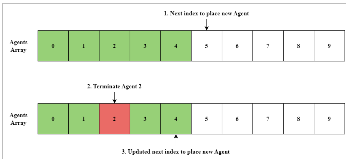
Figure 4.1: Using alive agents count to place new agent, which revealing a significant bug
