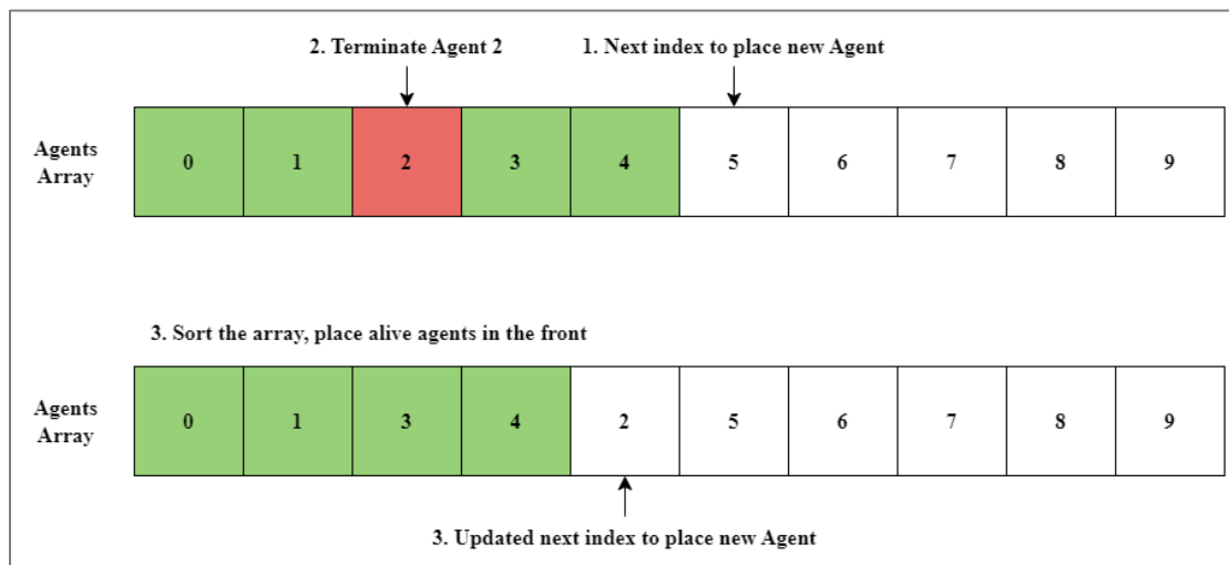
Figure 4.2: Original design for managing the agent array: sorting the array using CUDPP's radix sort to place alive agents in the front and dead agents at the end of the array
