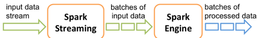
Figure 2.4 Spark Streaming workflow
