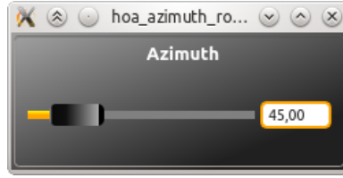
Figure 14: hoa_azimuth_rotator compiled using faust2jaqt script. The slider Azimuth allows to choose the azimuth angle of rotation, around the z -axis.
