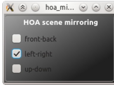
Figure 12: hoa_mirroring compiled using faust2jaqt script. The check-boxes allows to select the mirror transformations among: left-right , front-back or up-down .
