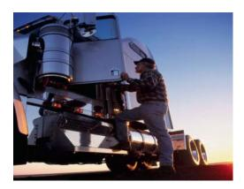
Always use three points of contact when entering and exiting the cab!
