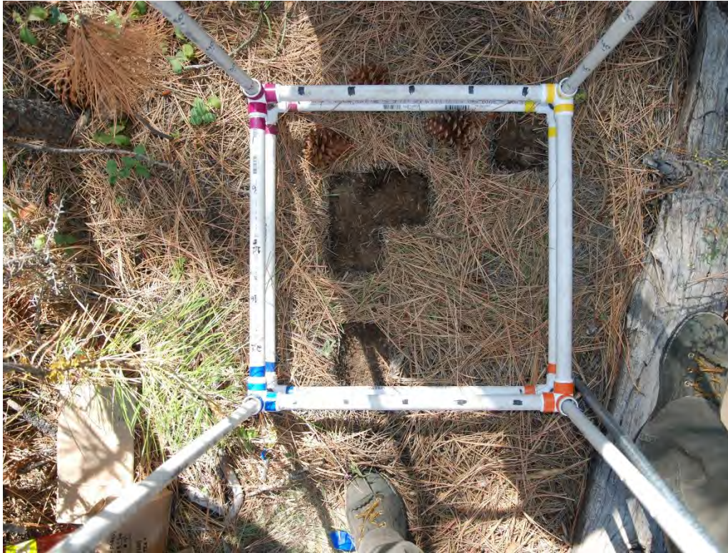
Figure 10: Photo of 0-10 cm stratum at the Sycan Forest site following sampling of the five randomly-sampled 10x10x10-cm voxels.
