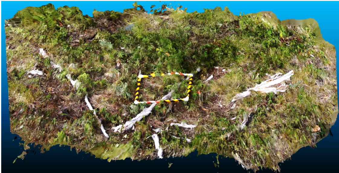
Figure 9. Close-range photogrammetry scan with a 2D frame representing the footprint of a clip plot, Lubrecht Experimental Forest.
