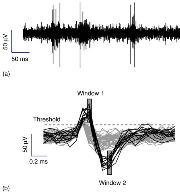
Fig. 4. (a) Sample of multi-unit spike activity recorded by the neurochip from M1 while the animal moved about the home cage. (b) Operation of the time–amplitude window discriminator. Waveforms crossing the trigger level are overlaid. The accepted waveforms (dark) are those that pass through the two user-positioned time–amplitude windows (gray boxes).
