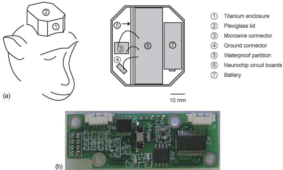
Fig. 1. (a) Components of the implant. All parts are enclosed in a titanium casing and mounted on the head. (b) Photograph of a neurochip circuit board. Actual size: 1.2 cm × 5.4 cm.
