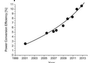
Figure 1. OPV Power Conversion Efficiency (Scharber, 2013).
