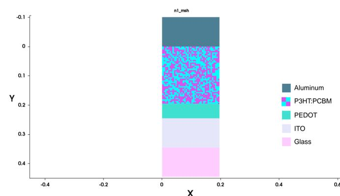
Figure 2. P3HT:PCBM bulk heterojunction semiconductor.
