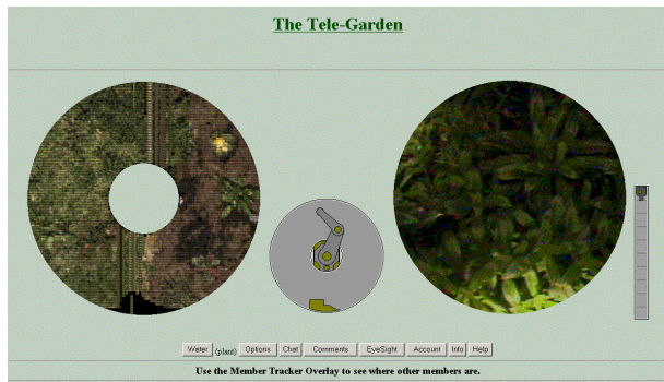
Figure 2. The World Wide Web interface to the Telegarden. The image on the left provides a composite view of the entire garden region and the image on the right is captured by the camera on the end of the robotic arm. Users can move the robotic arm by clicking on locations in the various images.
