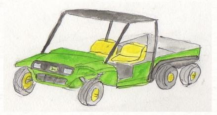
John Deere Gator TH 6x4 B99 Biodiesel, year round, no additives 18 HP, 1200 lbs box load Significantly reduced tailpipe emissions
