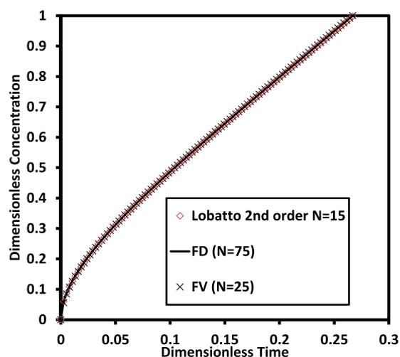
**Figure 1.** Comparison of Lobatto IIIA 2<sup>nd</sup> order method with converged Finite Difference and Finite Volume.
