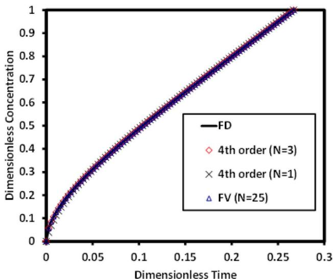
**Figure 2.** Comparison of Lobatto IIIA 4<sup>th</sup> order method with Finite Volume and with Finite Difference using constant diffusion coefficient and galvanostatic charging.
