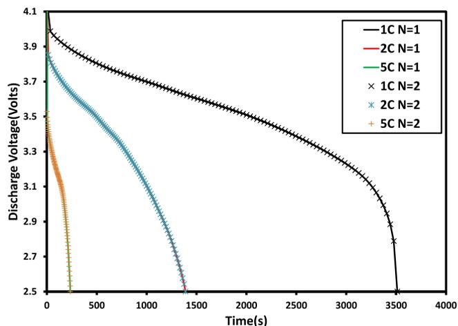
**Figure 7.** P2D model coupling with Lobatto IIIA 4<sup>th</sup> with  $N = 1$  and  $N = 2$  internal nodes showing convergence.
