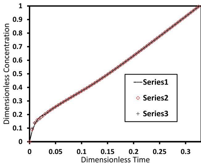
**Figure 5.** Convergence of the 4<sup>th</sup> order Lobatto method with concentration dependent diffusion coefficient given by  $f(c) = 0.1 + 9.9 * C$  and galvanostatic charging current.
