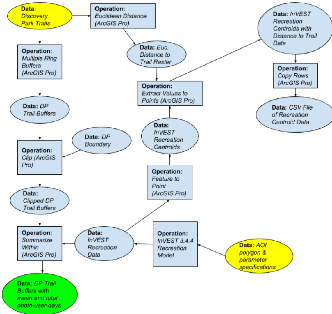
Figure 18. Operations flow diagram for buffer and Euclidean distance analysis. Input data shown here in yellow, output data products shown here in green.
