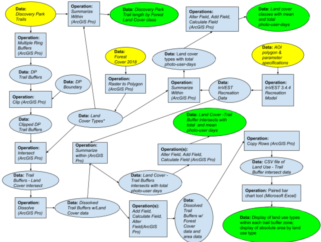
Figure 19. Operations flow diagram for land classification zone/ analyses. Input data shown in yellow, output data products shown in green.
