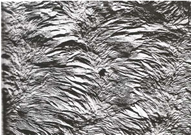
Ringed spherulites of poly(trimethylene glutarate) observed in the optical microscope between crossed polarizers (Keller 1959)
