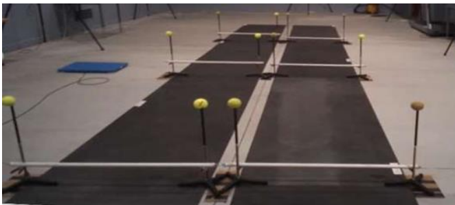
Figure 1: View from the start of the obstacle course. Six obstacles spaced 3 m apart. Participants walk the right side (12 m) to the end of the walkway, come back on the left side, and repeat for 2 minutes.
