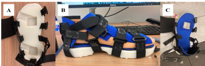
Figure 1: Ultrashoe design. (A) Polyurethane molded shoe and straps. (B) Prosthetic foot secured for visual. (C) Ultrashoe with load cells, ultrasound probe, insole liner, and gel pad.
