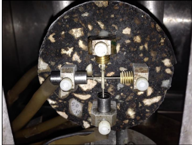
Figure B.3 Asphalt Mixture Sample Mounted with LVDTs
