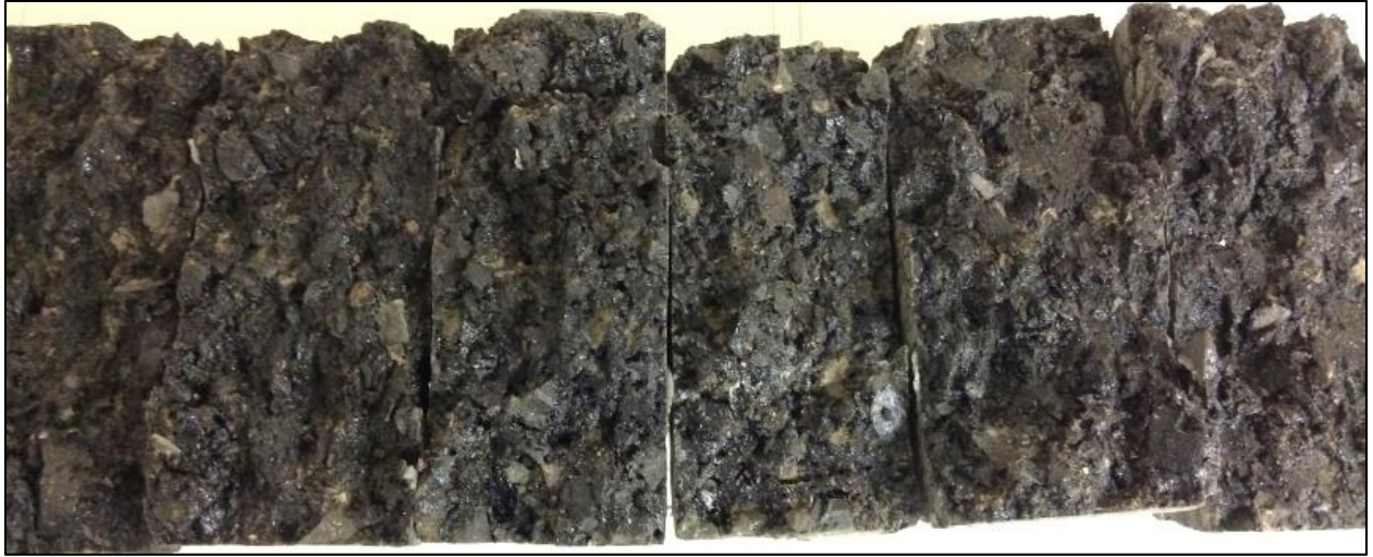
Figure B2.4 HMA Samples after IDT Fatigue Test
