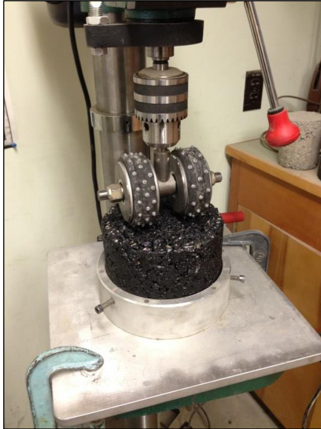
Figure B.15 Studded Tire Wear Simulator with Gyratory Sample
