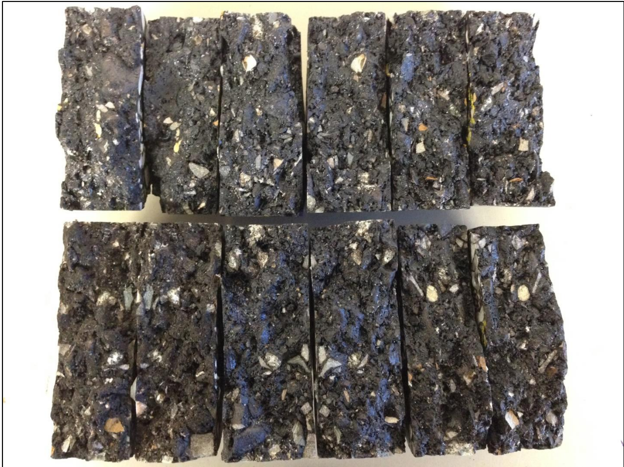
Figure B1.10 1/2" (Top Row) and 3/8" (Bottom Row) Mixes after IDT Thermal Cracking Tests
