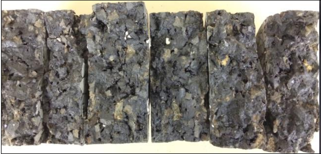
Figure B2.10 SMA Samples after IDT Thermal Cracking Tests
