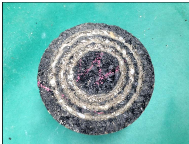
Figure B.2 Field Core Sample after Studded Tire Simulation
