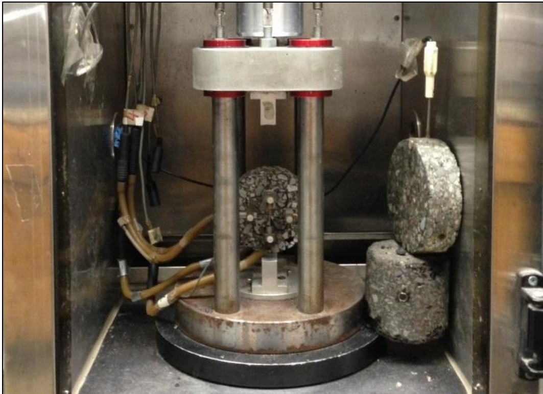
Figure B.4 IDT Test Machine Setup
