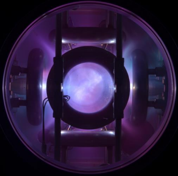
FIG. 3. Time integrated raw visible light image of plasma from a high \beta shot (#15640).
