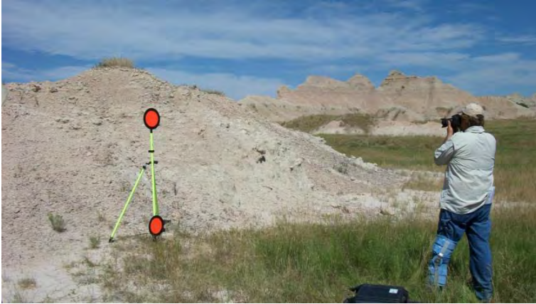
Photo 2. Dr. Larry Stetler from the South Dakota School of Mines and Technology taking stereo pair images of an erosion study site in BADL using photogrammetry techniques (photo by Emily French, SD School of Mines and Technology, 2011).
