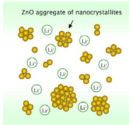
Fig. 11. A schematic showing the impact of lithium ions on the growth of ZnO aggregates.
