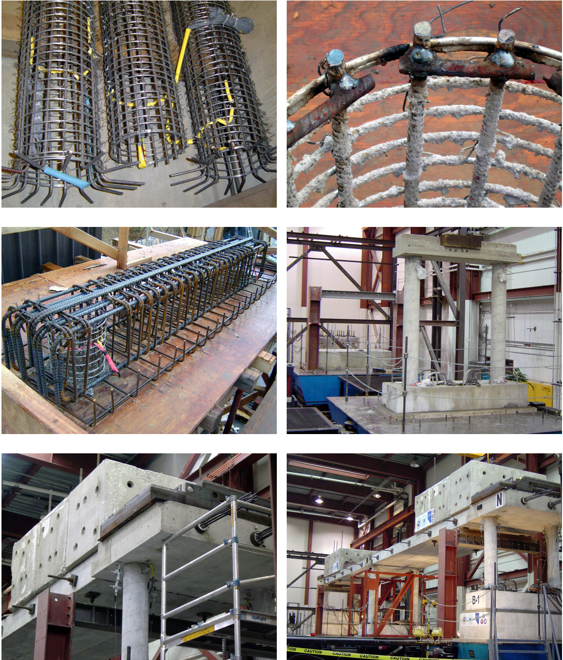
Figure 2.3: Photographs of construction sequence, including: a) column cages, b) column welds, c) beam cages, d) bent assembly, e) external slab masses, and f) final pre-test specimen
