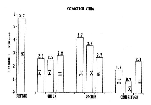
FIGURE 3. Testing time for each method of extraction.
