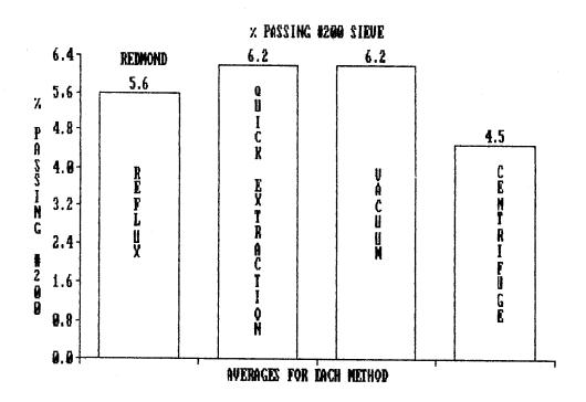
FIGURE 15. Average percent passing the #200 sieve for the Redmond samples for each extraction method.
