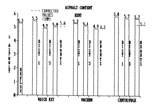
FIGURE 5. Asphalt percentages for the Kent samples for each extraction method.
