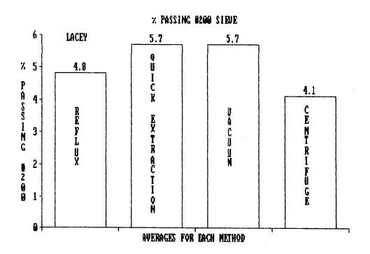
FIGURE 13. Average percent passing the #200 sieve for the Lacey samples for each extraction method.
