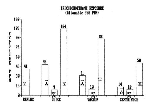
FIGURE 2. Exposure level for each method of extraction.
