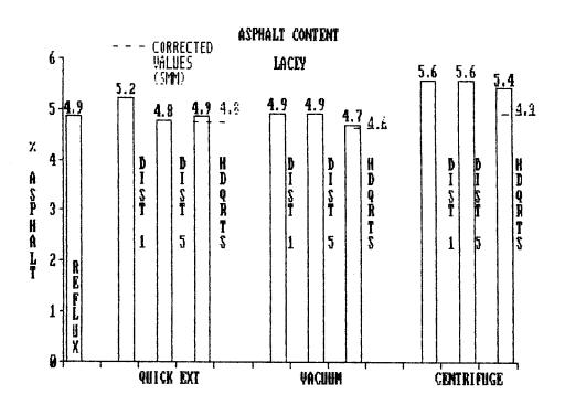
FIGURE 4. Asphalt percentages for the Lacey samples for each extraction method.
