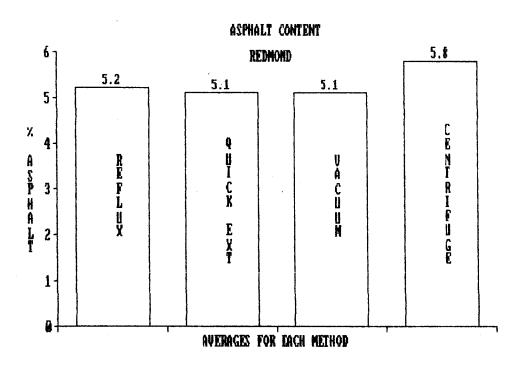
FIGURE 12. Average asphalt content for the Redmond samples for each extraction method.
