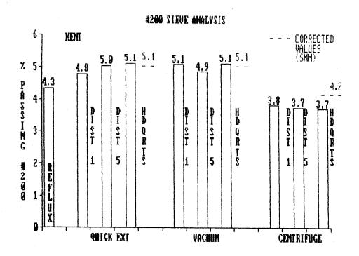
FIGURE 8. Percent passing the #200 sieve for the Kent samples for each extraction method.
