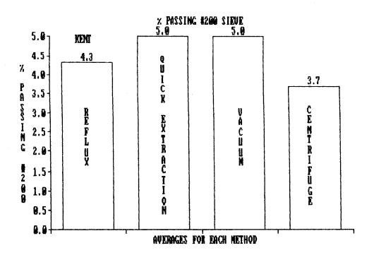
FIGURE 14. Average percent passing the #200 sieve for the Kent samples for each extraction method.
