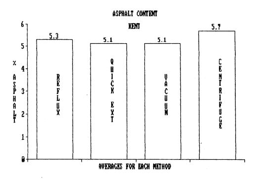
FIGURE 11. Average asphalt content for the Kent samples for each extraction method.
