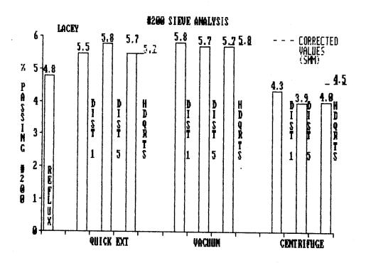
FIGURE 7. Percent passing the #200 sieve for the Lacey samples for each extraction method.
