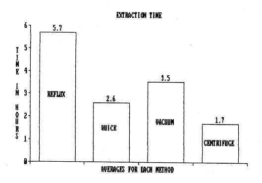
FIGURE 17. Average testing time for each method of extraction.
