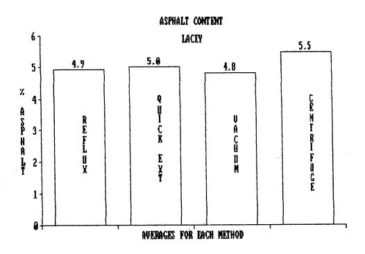
FIGURE 10. Average asphalt content for the Lacey samples for each extraction method.
