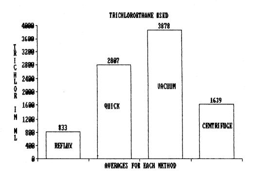
FIGURE 16. Average trichloroethane usage for each extraction method.
