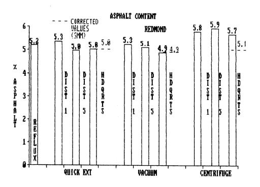
FIGURE 6. Asphalt percentages for the Redmond samples for each method of extraction.
