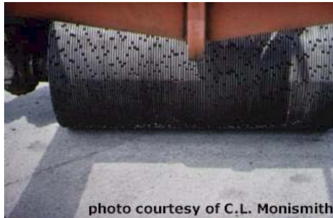
Figure 7. Diamond grinding cutting head.
