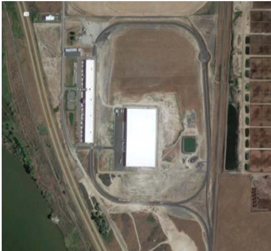
Figure 8. Aerial View of Railex Facility in Wallula, WA. Loop Track Allows 19 Cars to Enter the Building on the Left for Loading. Photo from Google maps.
