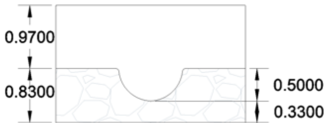
Figure 2 Cross section of a trench dug for DGC.
